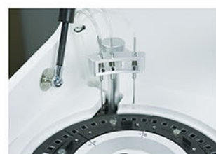
Washing Probe Independent 3 -step washing system.
