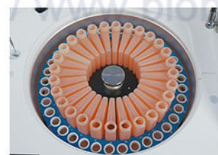
Reagent Tray Refrigerated tray with independent switch.
